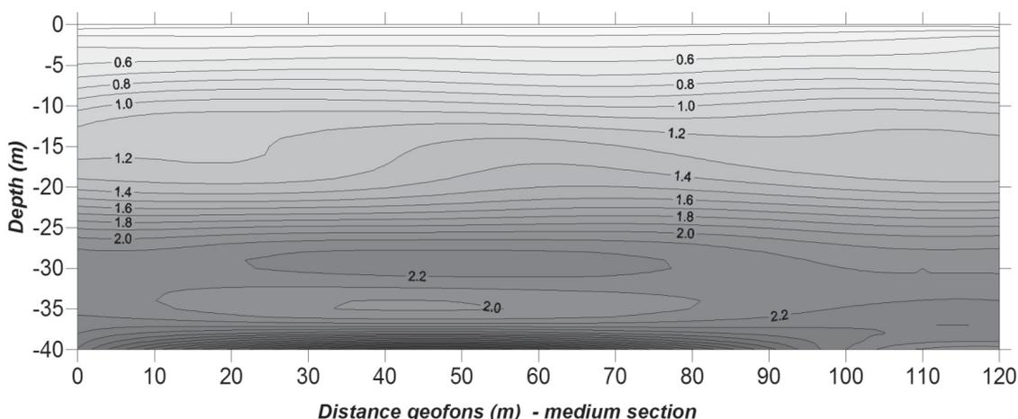
FIGURE 6. Mean seismic section showing velocities.
