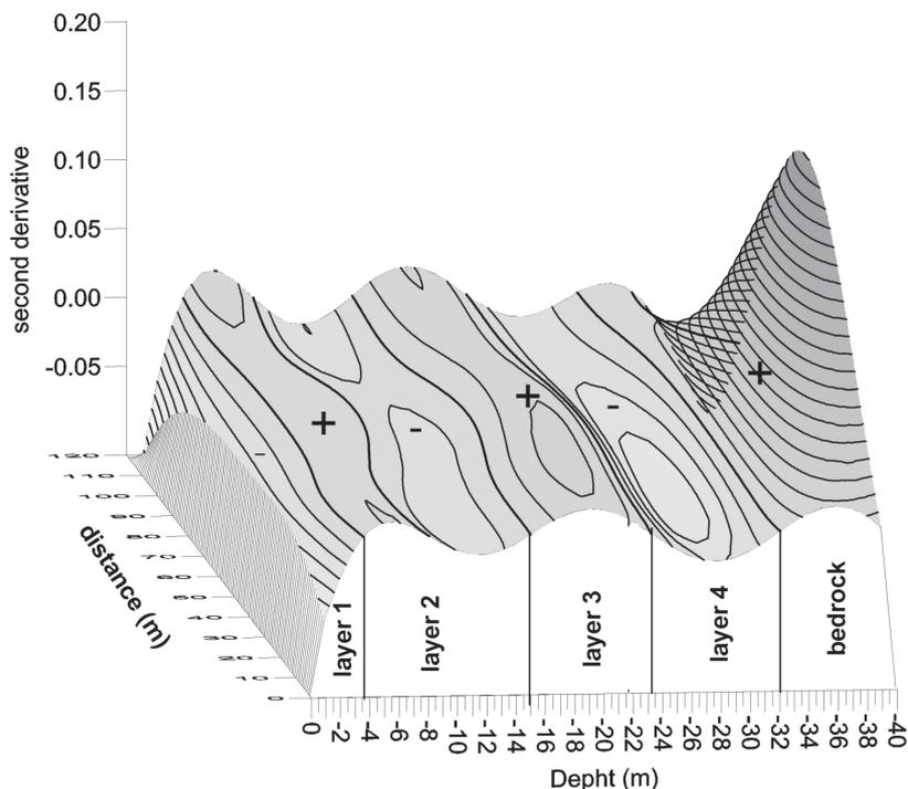
**FIGURE 8.** Perspective view of the second derivative of the mean section and delimitation of the hypothetical thickness of compactness, where the iso-value curve of the second derivative is zero.
