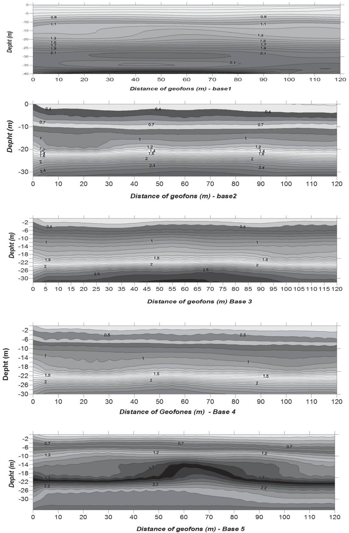
FIGURE 5. Seismic sections showing, in detail, the increase in wave velocity with depth.
