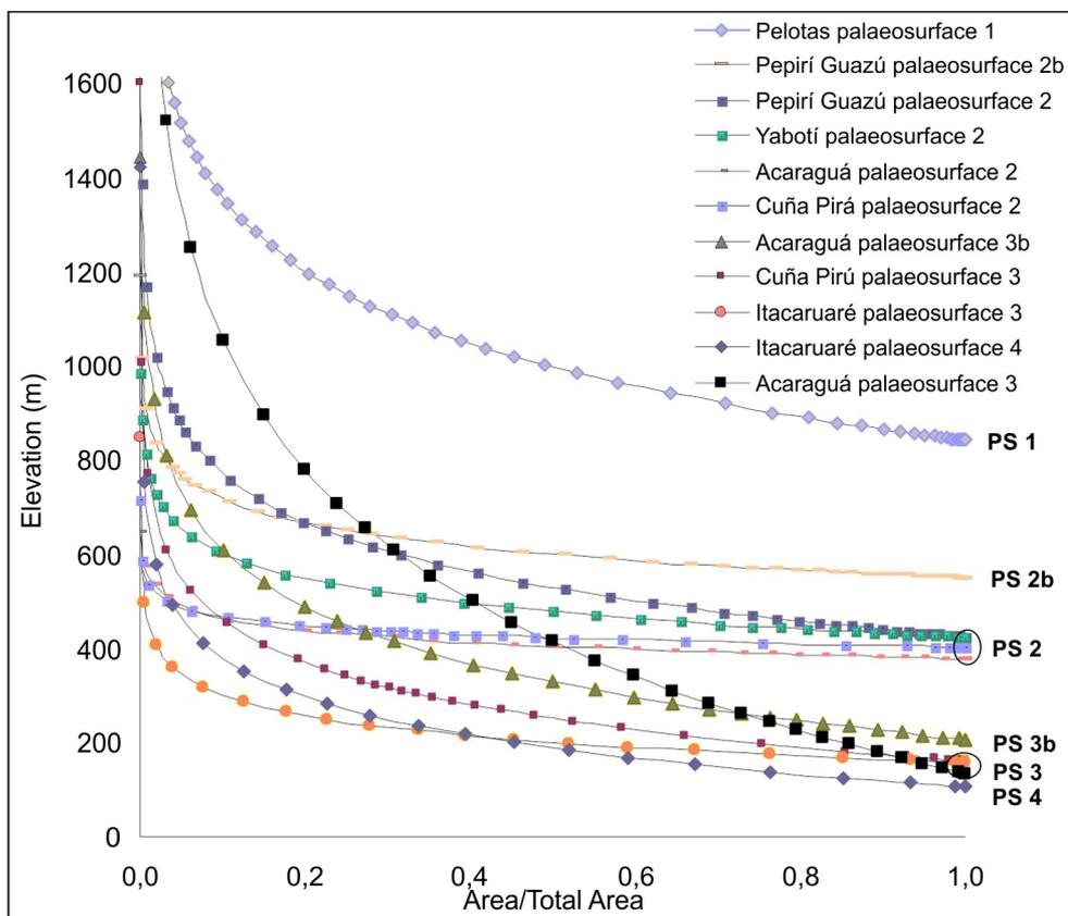
**FIGURE 6.** Modeled hypsometric curves, with elevation values (H) and cumulative areas (A), re-scaled to 1: area above altitude H divided by the total area. Predicted base level elevations allow grouping hypsometric curves and defining three main palaeosurfaces and several secondary ones.
