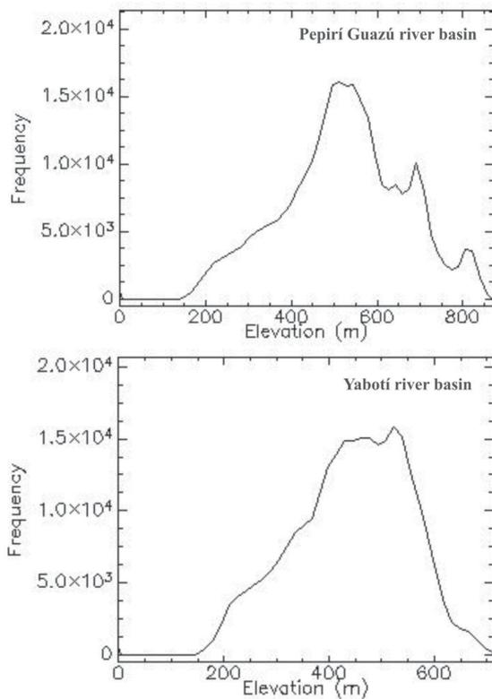
**FIGURE 2.** Frequency histograms of Pepirí Guazú and Yabotí river basins, obtained from SRTM (90 m) - DEM data and calculated by using ENVI 4.0 software.
