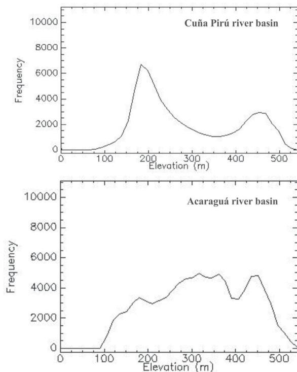
**FIGURE 3.** Frequency histograms of Cuña Pirú and Acaraguá river basins, obtained from SRTM (90 m) - DEM data and calculated by using ENVI 4.0 software.
