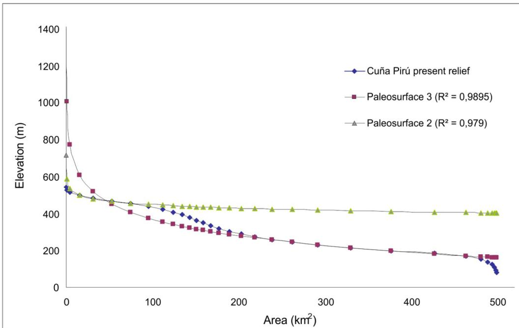
**FIGURE 5.** Hypsometric curves of the Río Cuña Pirú basin. Diamond plots represent the present relief. Hypothetical hypsometric curves obtained from regression analyses, by fitting the low gradients segments, correspond to triangle and square plots. They represent palaeosurfaces and the relatively flat segments are considered as their remnants.
