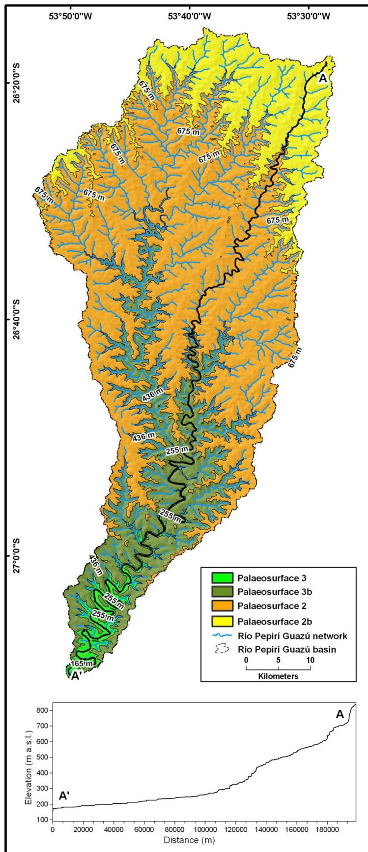
**FIGURE 9.** SRTM-DEM-based map of paleosurfaces in the Río Pepirí Guazú basin. The simulated hydrographic network is also represented. In the insert, the longitudinal profile extracted from the main collector of the basin is shown.
