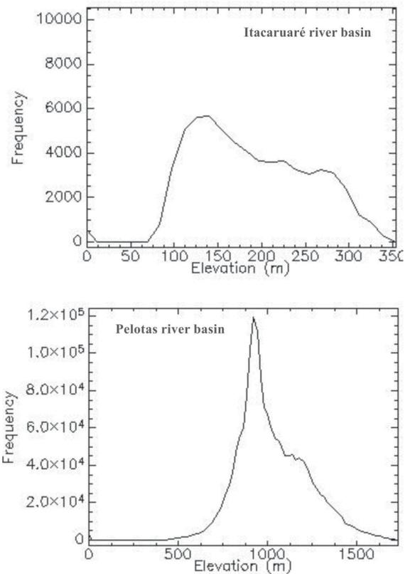
**FIGURE 4.** Frequency histograms of Itacaruaré and Pelotas river basins, obtained from SRTM (90 m) - DEM data and calculated by using ENVI 4.0 software.
