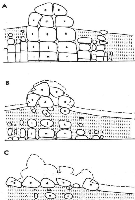
**FIGURE 9.** Stages in the collapse of a domical tor. (a) Initial phase in the dismantling of the tor group, with partial removal of the weathered debris; (b) progressive collapse of the tor as a result of the washing out of the weathered materials; (c) superficial distribution of the remaining corestones. From Thomas, 1965.
