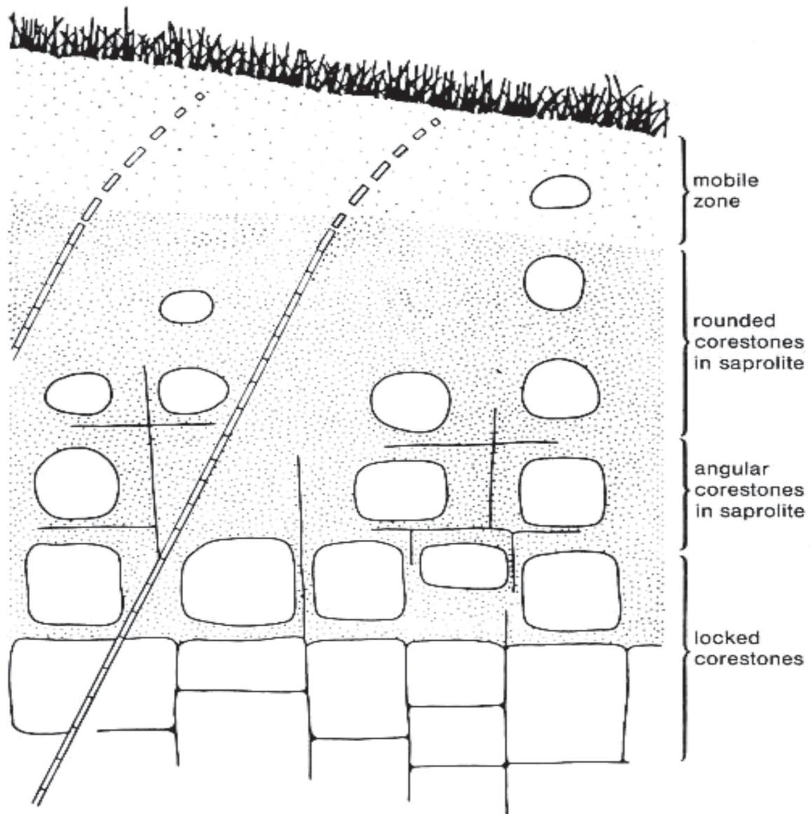
**FIGURE 6.** Granite weathering. A typical section of weathering in granites. Saprolite is an in-situ weathered rock, as indicated by the non-removed quartz veins. The alteration is iso-volumetric. Regolith is a term that includes all unconsolidated materials near the surface of the Earth, including saprolite. From Ollier, 1990.
