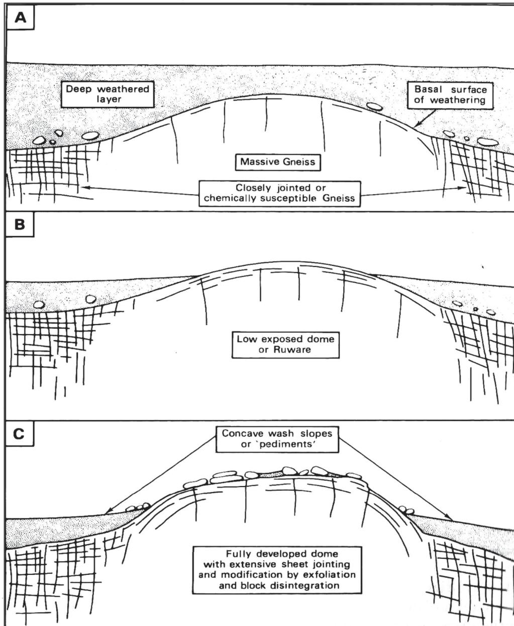
**FIGURE 13.** The development of ruwares and low domes by differential deep weathering and subsurface stripping of the deep weathered layers. From Small, 1978.
