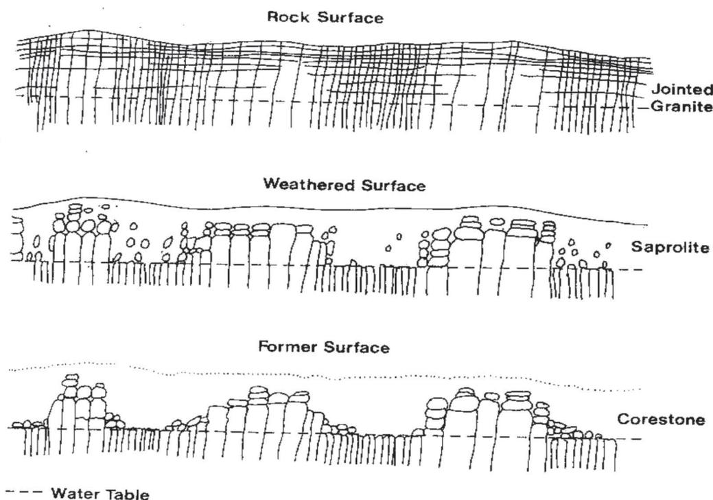
**FIGURE 7.** Corestone and tor development due to deep weathering and subsequent denudation, with finer, weathered material removal. From: Linton, 1955; see Fairbridge, 1968.
