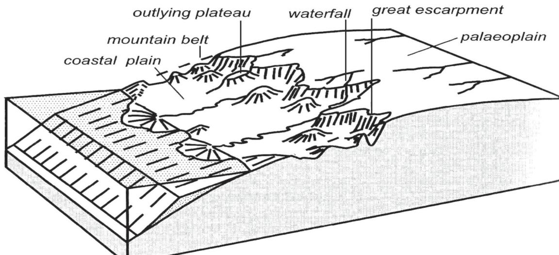
**FIGURE 15.** In passive continental margins, a large and continuous escarpment is developed by headward erosion from the coastal plain, degrading a former paleoplain, usually an etchplain, developed during previous stages of tropical climate with deep chemical weathering. The position of the escarpment is noted by waterfalls along a very steep boundary. From Ollier and Pain, 2000.
