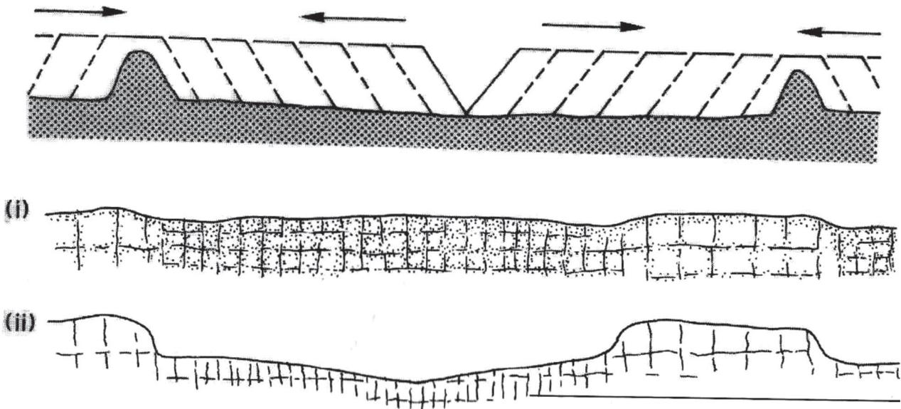
**FIGURE 10.** Formation of inselbergs and bornhardts. Upper figure: Inselbergs resulting from long-distance scarp retreat; lower figure (i) initial stage of etching of differentially jointed bedrock; (ii) final stage after removal of the weathered cover. From Twidale, 2007b.
