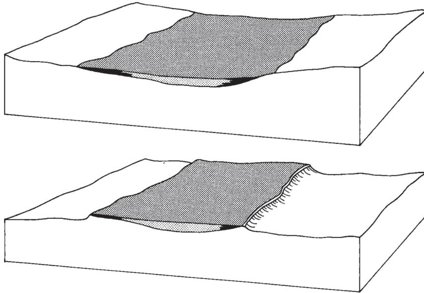
**FIGURE 16.** Duricrusts and inversion of relief. From Ollier, 1991. In the top figure, ferricretes are precipitated on lower slopes and valley bottoms. The bottom figure shows the inversion of relief, producing a ferricrete-capped mesa or tableland.
