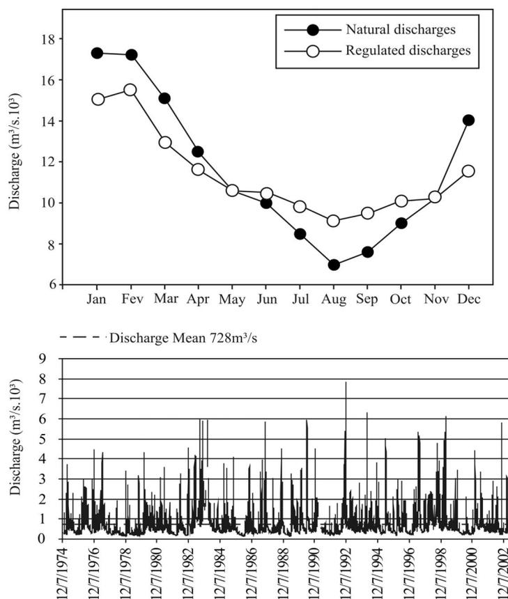
**FIGURE 3.** Upper – Paraná River annual hydrograph: flow regulation flattened the high-low water peaks if compared with natural discharge. Lower: Ivaí River annual hydrograph: Flood peaks reaches more than 10 times mean water level.
