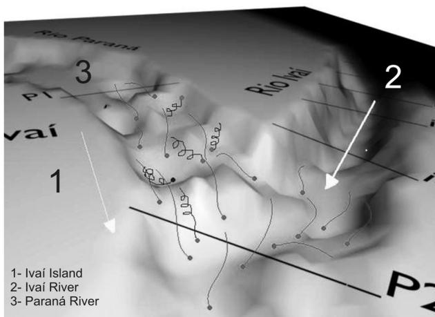
**FIGURE 6.** 3-D Diagram of the Ivaí and Paraná River confluence constructed from detailed echo-bathymetric survey. Note sand bar morphology in the Paraná River channel upstream confluence. Arrows indicate horizontal and vertical vortex flow.
