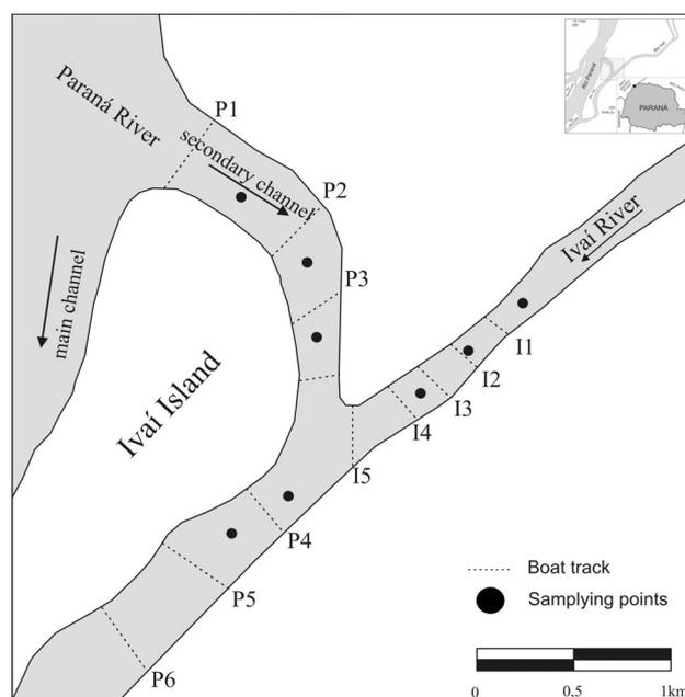
**FIGURE 4.** Localization of echo-sounding and ADCP profiles (interrupted lines) and bedload sampling points.
