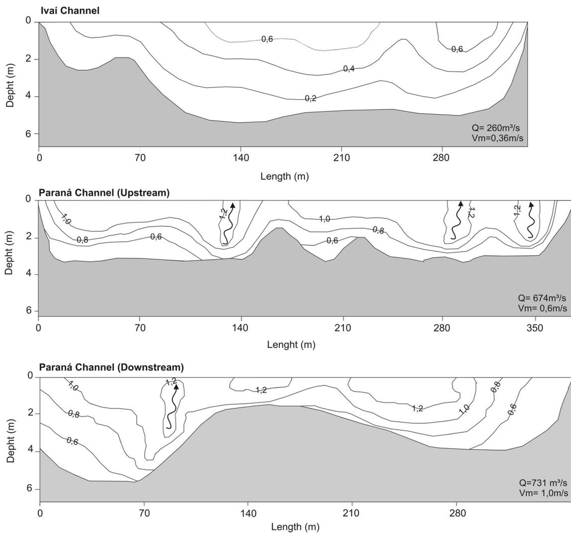
**FIGURE 7.** Flow velocity distribution in channel cross sections at confluence area obtained by ADCP. A. Ivaí River and B. Paraná River – vertical and sinuous arrows mark upwelling flows (See Figure 4 for localization).
